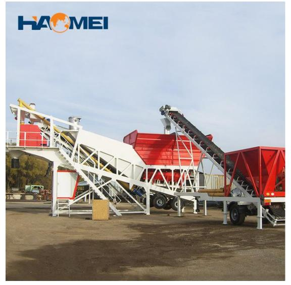
YHZS75 batching plant belongs to a large-sized one among four models with capacity of 75  $\,\mathrm{m}^3/\mathrm{h}$ . It is completely mobile and travels as a single load of freight including dust collection, saving you transportation cost.
