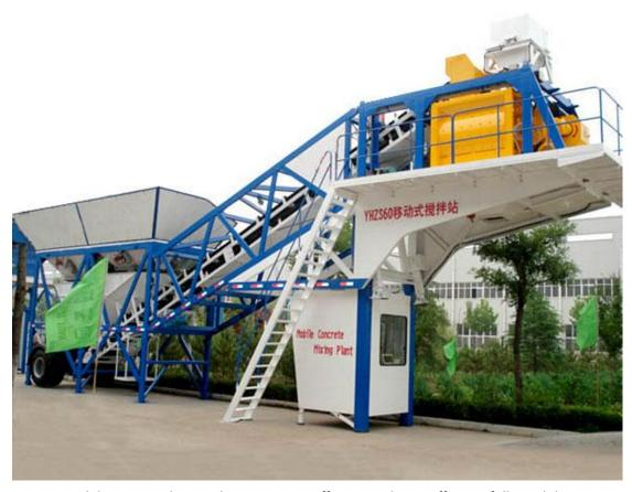
YHZS60 mobile mixing plant is the most time efficient and cost-effective fully mobile concrete batch plant available today. All the parts are installed on a transport chassis. At the job site, it can be operational in less than 4 hours.
