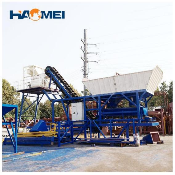
YHZS25 mobile concrete plant is an all-in-one concrete plant. By absorbing new technologies from overseas and domestic, the mobile concrete batching plant has such characteristics as accurate weighing, even and efficient mixing, fast and clean delivery, etc.
